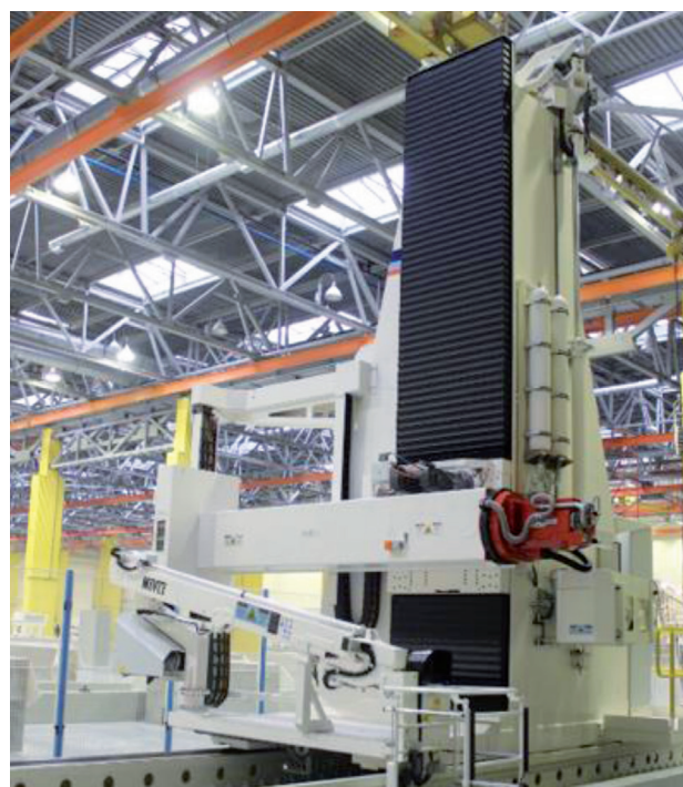
Fig. 3. Automated drilling machine with numerical control
