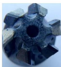
Fig. 2. MAPAL replaceable-head reamer (Ø14 mm)
