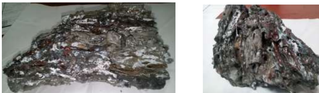
Fig. 4. Magmatic mixture of fused silica and slag with various content of residual silicon oxide and reduced silicon
