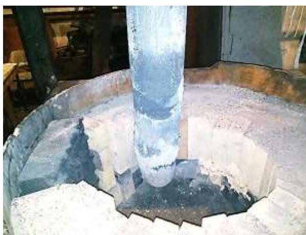
Fig. 6. The structure of the melting bath of the furnace with a 200 kVA transformer: 1 – electrodes; 2 – initial charge; 3 – softened charge zone; 4 – transition zone; 5 – wall lining; 6 – melt and silicon, carbide crust
