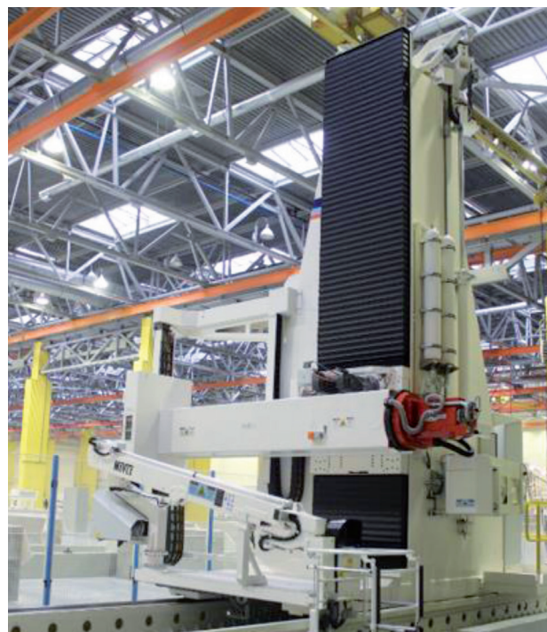
Fig. 3. Automated drilling machine with numerical control
