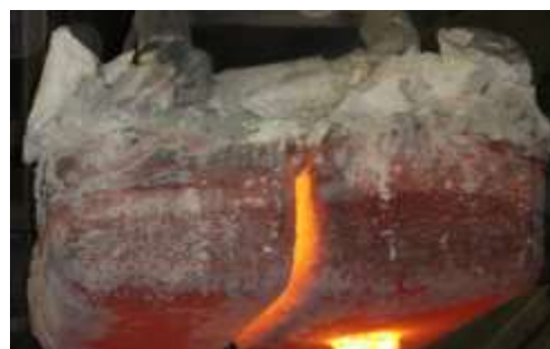
Fig. 2. Electrochemical local wear of the anodes along the edges around the perimeter
