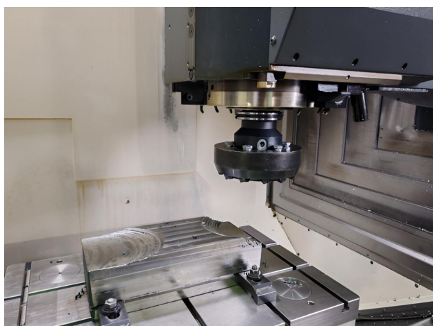
Рис. 3. Рабочая зона станка DMG DMU 80P Duo Block Fig. 3. Working area of the DMG DMU 80P Duo Block machine-tool
